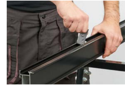
2. Build the sub-construction frame with corner piece
